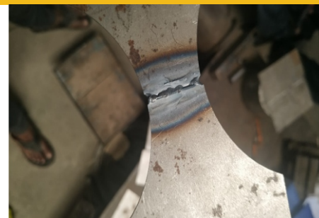
Pic: Tailor welded blanks
