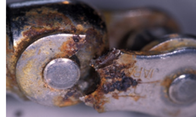
Pic: Corrosion in a linkage.
