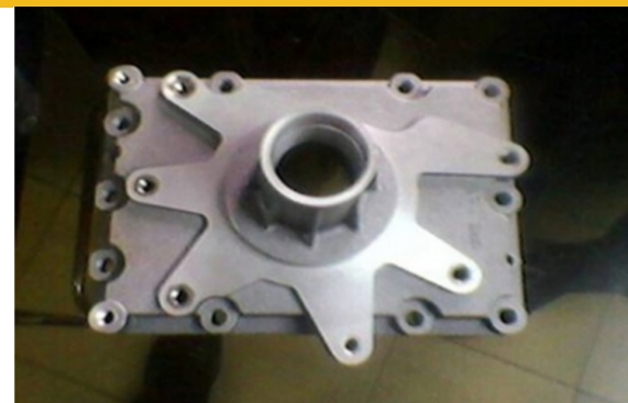
Pic: PTO cover for ape three-wheeler diesel engine used for leakage testing in Swagati Engineering Pvt Ltd.
