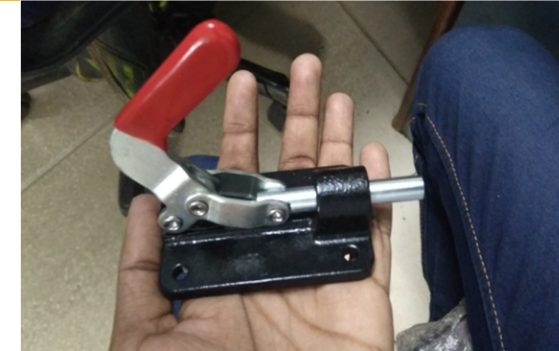
Pic: Illustration of toggle clamp (low duty).
