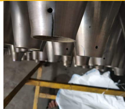
Pic: Shows crack formation along a fusion line
