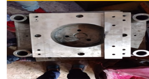
Pic: Die and insert assembly
